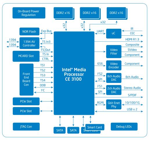
Figure 3 - The Intel® Media Processor CE 3100 Development Platform
