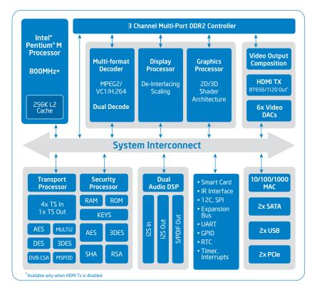
Figure 1 - Intel® Media Processor CE 3100 - Block Diagram
