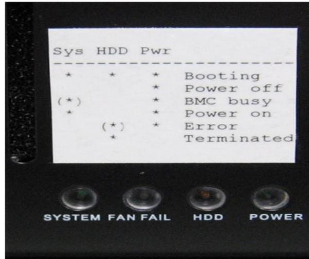
The label describes states for three LEDs, called Sys, HDD, and Pwr. ON
