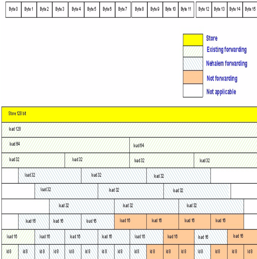
Figure 2-12. Store-Forwarding Scenarios of 16-Byte Store Operations
