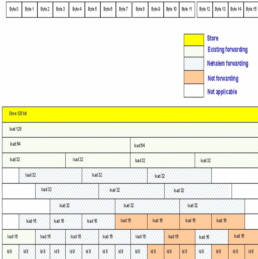
Figure 2-14. Store-Forwarding Scenarios of 16-Byte Store Operations
