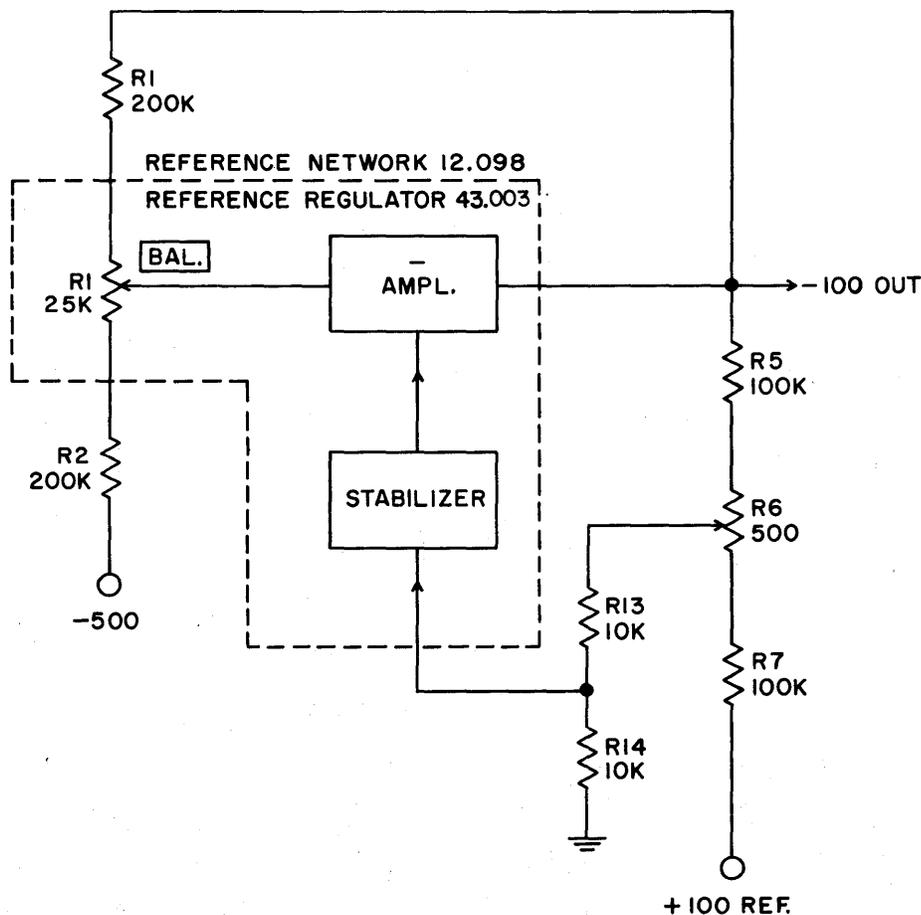
Figure 4. Block Diagram -100 Volt Reference Source.
