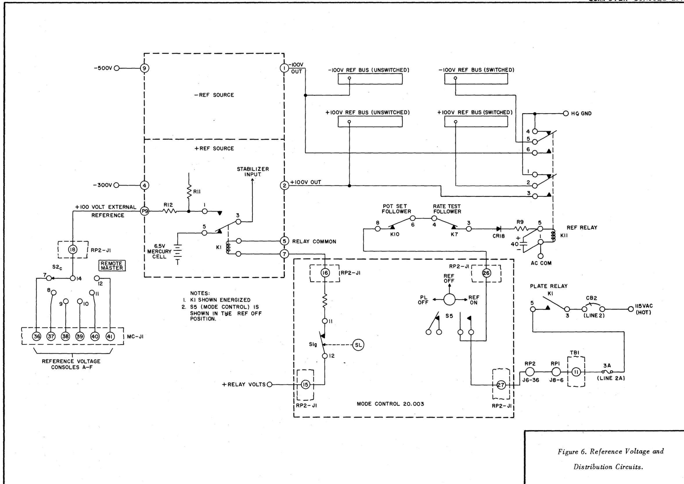
Figure 6. Reference Voltage and Distribution Circuits.
