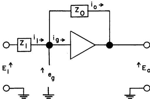
Figure 4. Multiplication by a Constant Coefficient.
