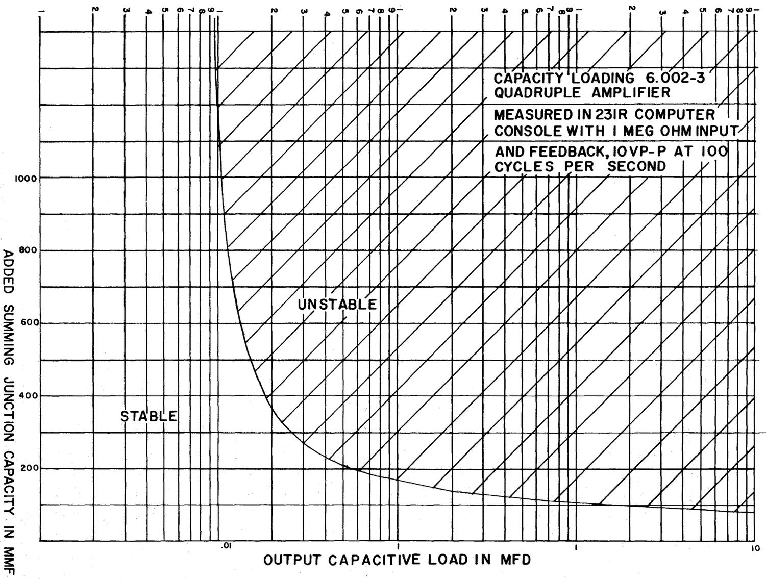
Figure 1. Capacity Loading, Amplifier 6.002-3
