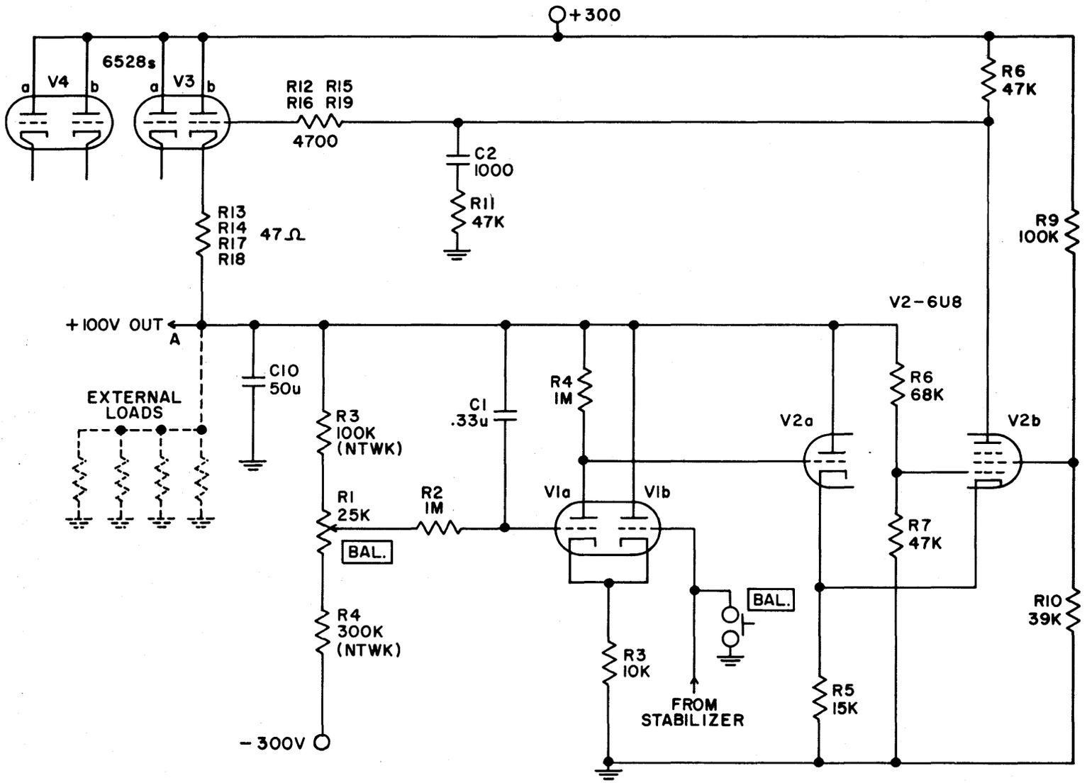
Figure 3. Amplifier Section of Reference Regulator 43.003.
