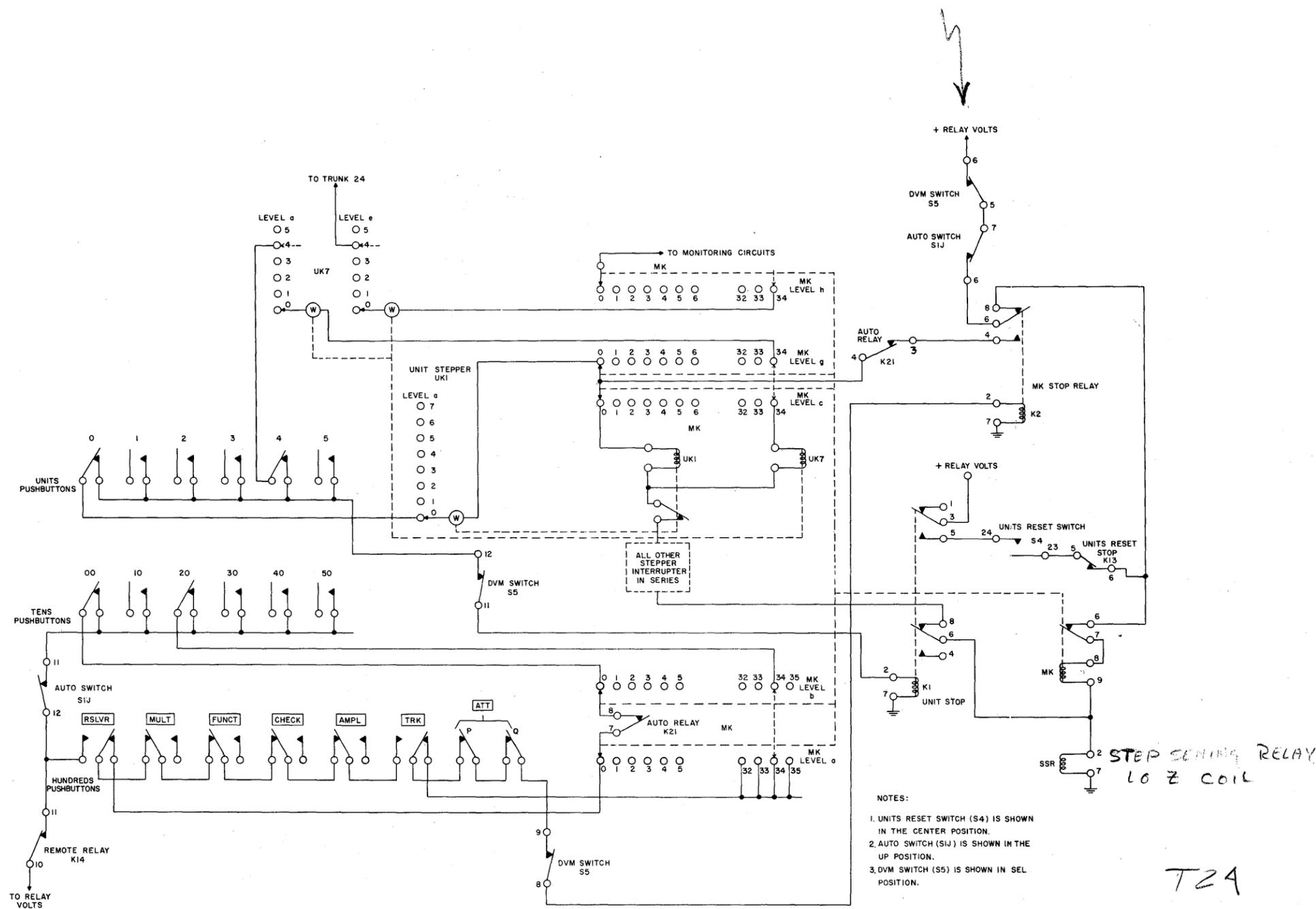
Figure 23. Manual Readout, Simplified Schematic.
