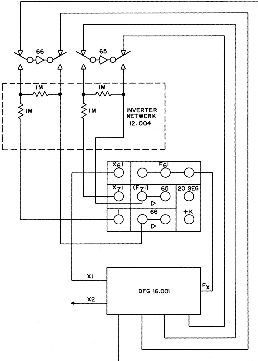
Figure 15. Diode Function Generator Connections.
