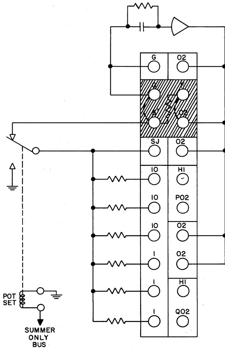
Figure 11. Summing Amplifier Connections.
