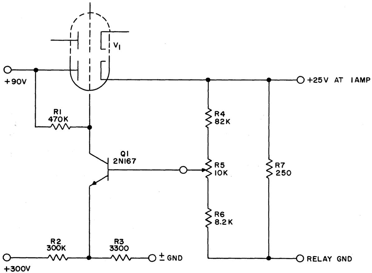
Figure 2. Power Supply 10.008, Simplified Schematic.
