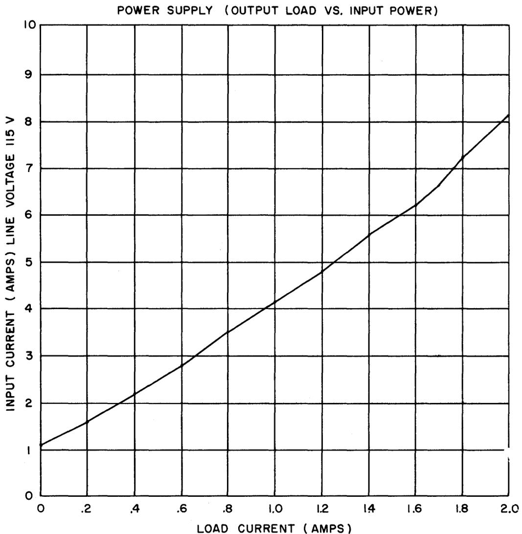
Figure 2. Input Power Requirements.
