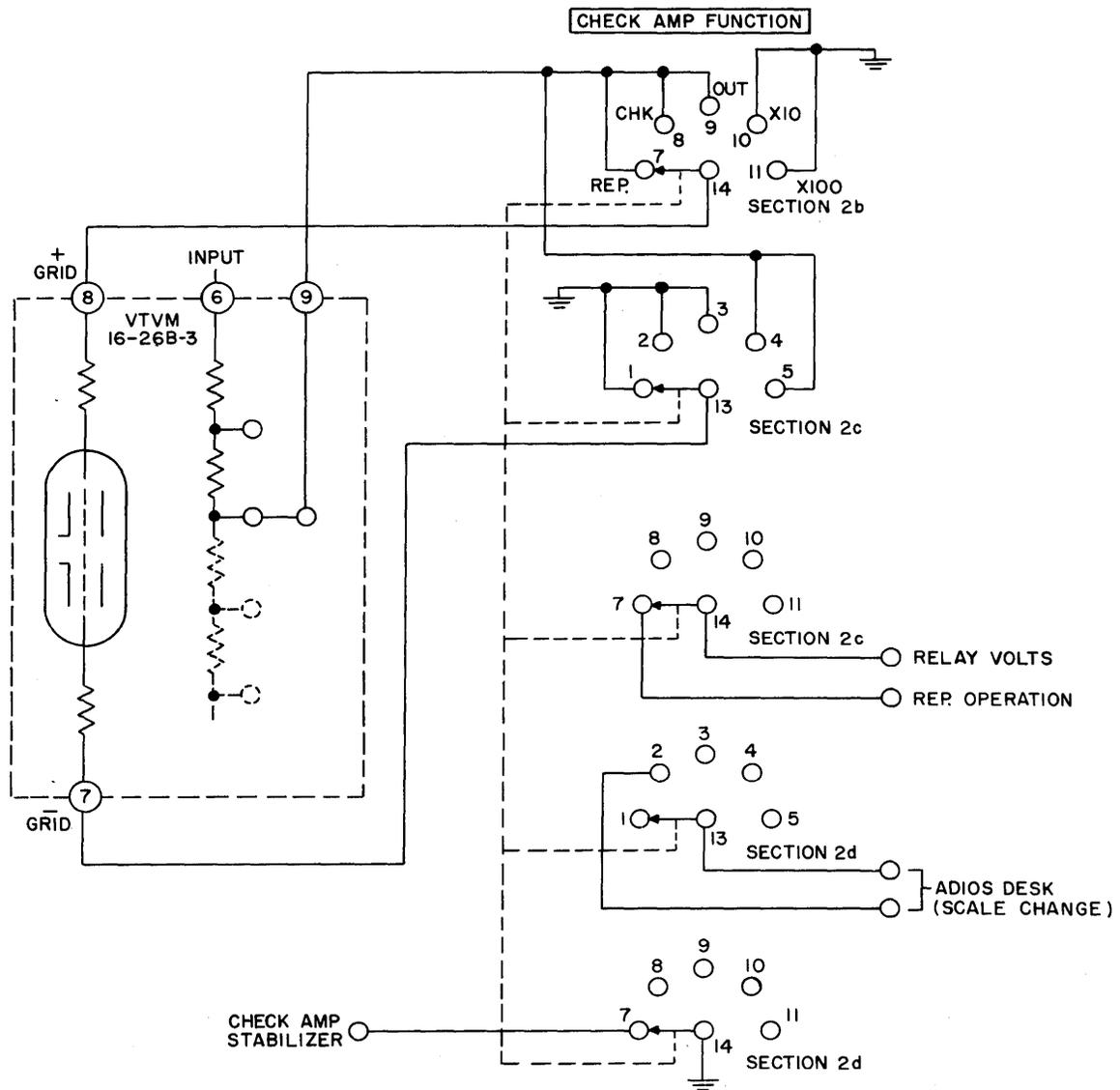
Figure 27. Check Amplifier Function Switch.
