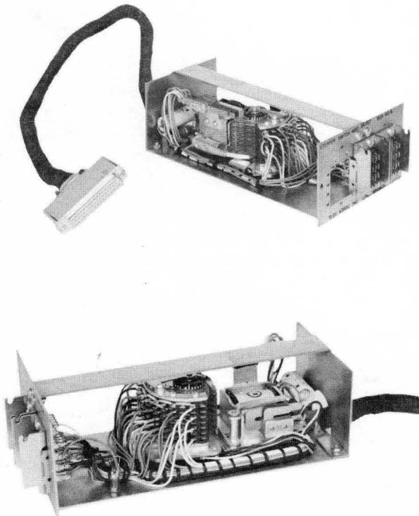
Figure 22. Typical Stepper Switch.
