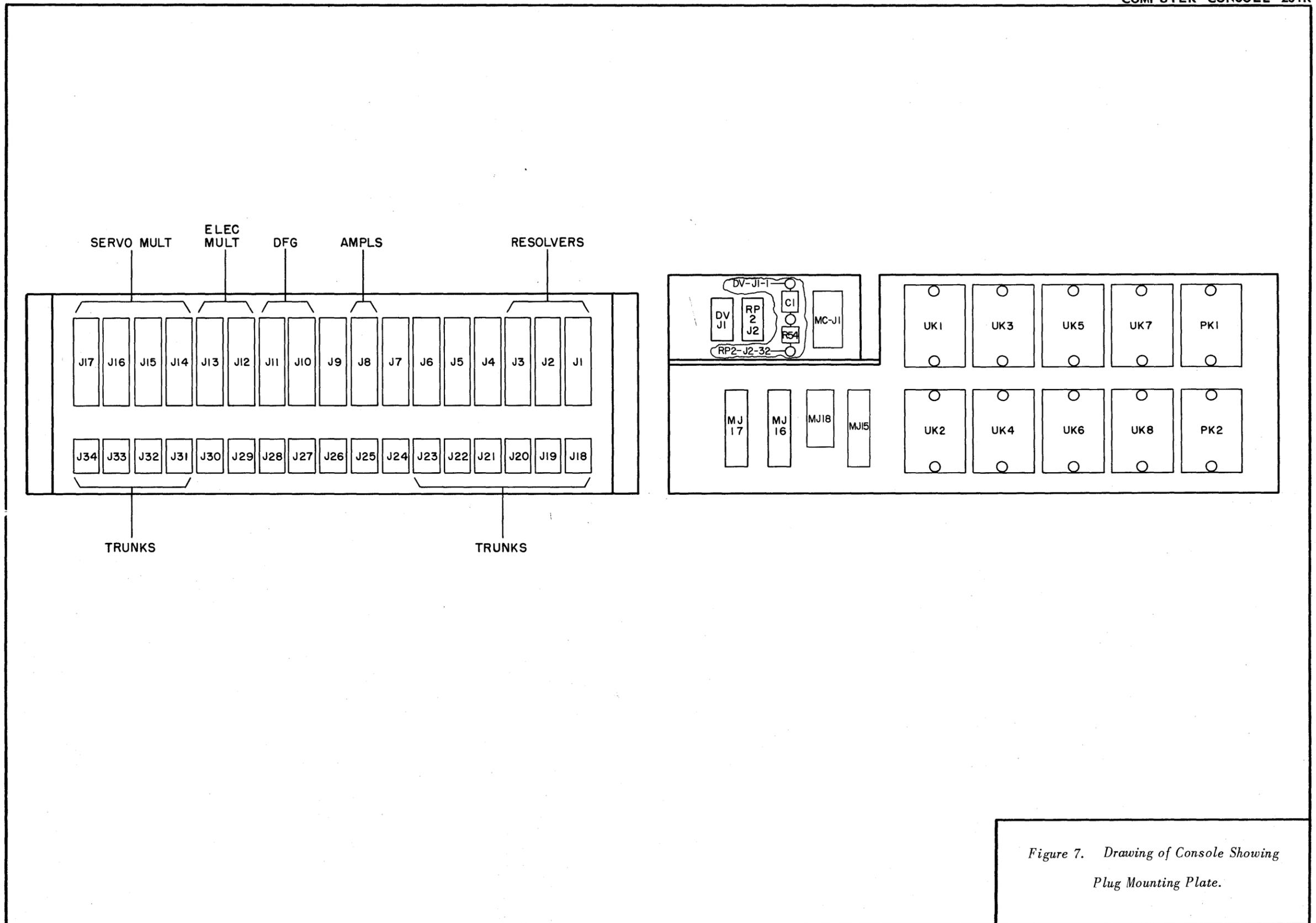
Figure 7. Drawing of Console Showing Plug Mounting Plate.
