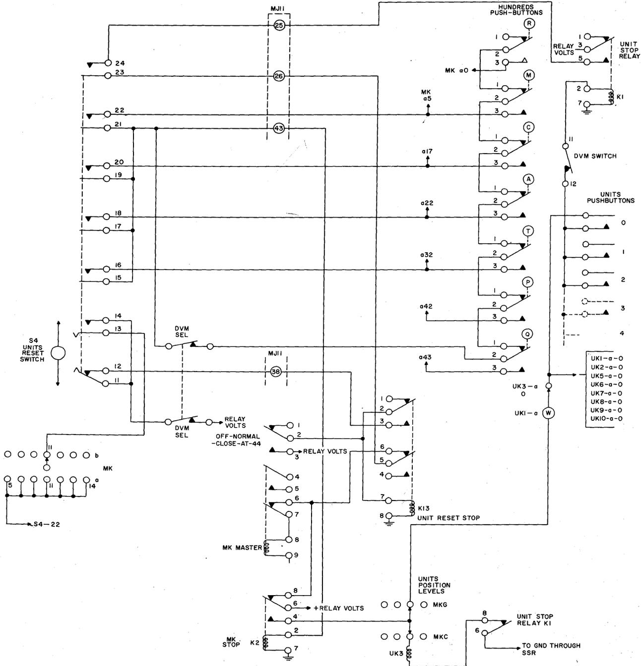
Figure 24. Units Reset Circuits, Simplified Schematic.
