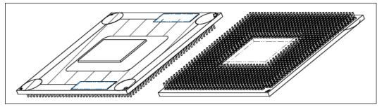
Figure 5. 3-D View of Top/ Bottom of rPGA988 4C/2CF Package for the 2nd Generation Intel® Core™ Processor Family Mobile
