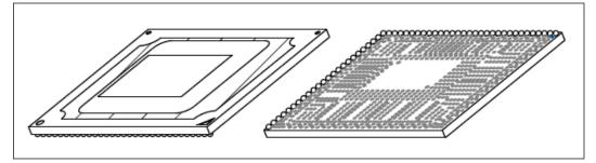
Figure 3. 3-D View of Top/ Bottom of BGA1023 4C/2CF Package for the 2nd Generation Intel® Core™ Processor Family Mobile
