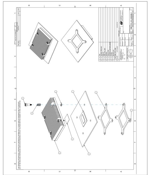
Figure 30. cPCI\* Reference Heatsink Assembly (Sheet 1 of 2)
