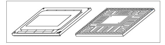
Figure 4. 3-D View of Top/ Bottom of rPGA988 2C Package for the 2nd Generation Intel® Core™ Processor Family Mobile
