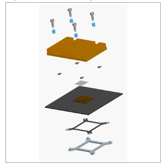
Figure 22. CompactPCI\* Reference Heatsink Assembly
