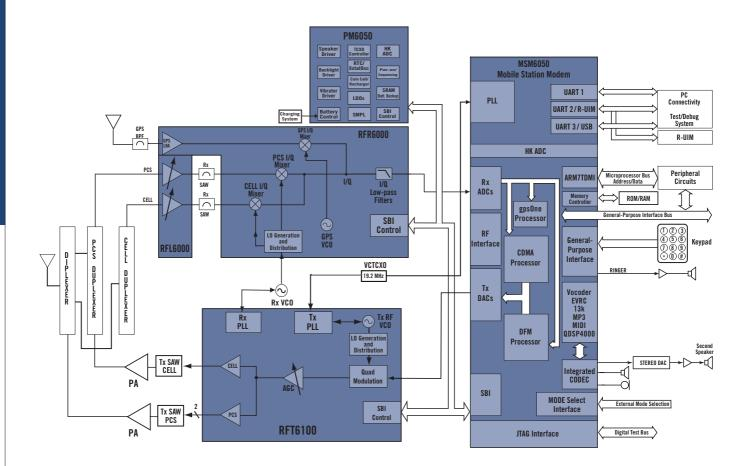
MSM6050 Chipset Solution Architecture Using QCT's radioOne Zero Intermediate Frequency (ZIF)
