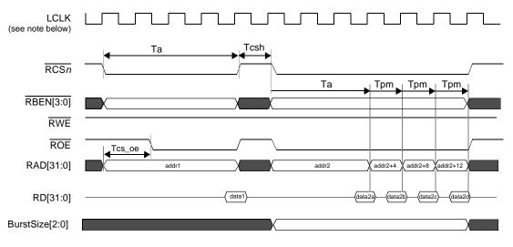
NOTE: The external clock LCLK is available only in synchronous mode (**mem\_stcfg**[S]=1). For *asynchronous* chip selects, the timing parameters are based on a separate internal-only clock.
