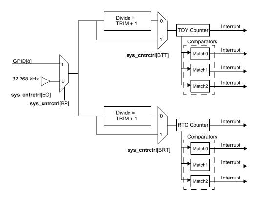
Figure 37. TOY and RTC Block Diagram
