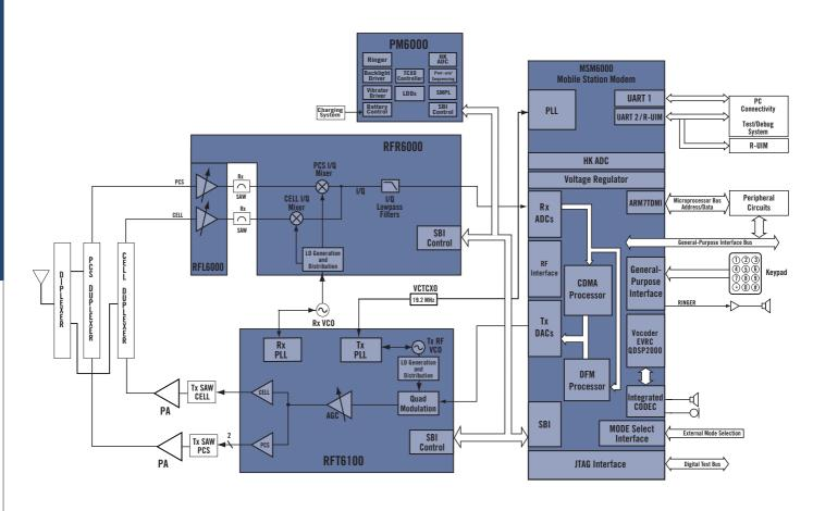
MSM6000 Chipset Architecture Using QCT's radiOne Zero Intermediate Frequency (ZIF)
