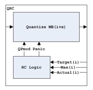
Macroblock level rate control is handled by the RC logic and the quantization logic.
