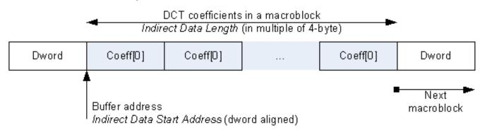
Each non-zero coefficient in the indirect data buffer is contained in a doubleword-size data structure consisting of the coefficient index, end of block (EOB) flag and the fixed-point coefficient value in 2's compliment form. As shown in *Common Indirect IT-COEFF Data Structure, index* is the row major 'raster' index of the coefficient **within a transform block** (*please note that it is not converted to 8x8 block basis*). A coefficient is a 16-bit value in 2's complement.
