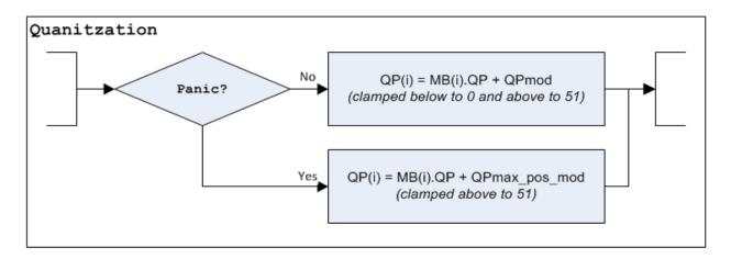
The signals QPmod and panic are generated by the RC logic based on data feedback from BSP. A flowchart of the RC logic is given below.
