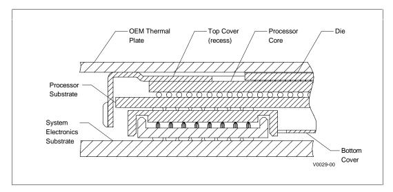
Figure 5.1 Mini-Cartridge Cross-Section View
