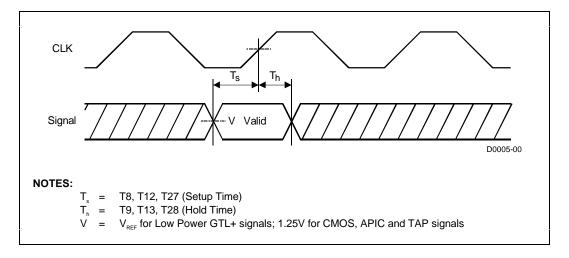
Figure 3.4 Setup and Hold Timings
