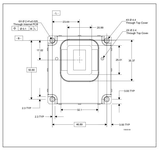
Figure 5.2. Mini-Cartridge Assembly, Top Cover (in mm)
