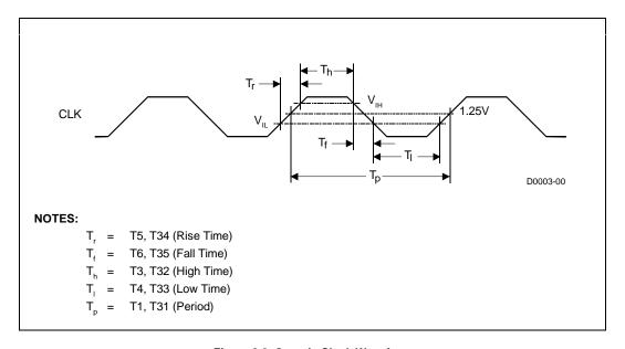
Figure 3.2 Generic Clock Waveform
