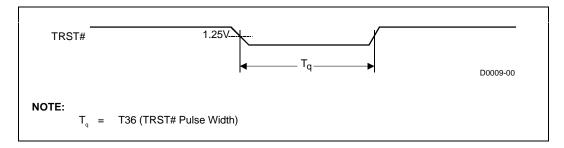
Figure 3.8 Test Reset Timings
