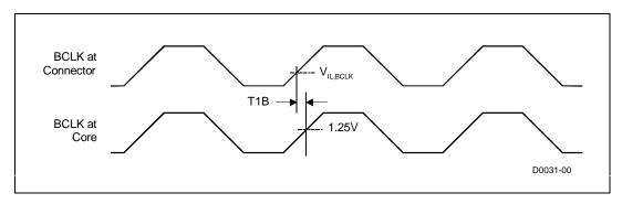
Figure 3.1 BCLK Connector to Core Offset
