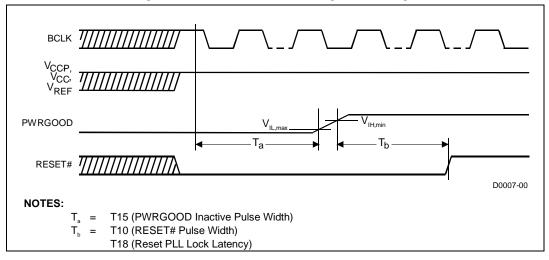
Figure 3.6 Power-On Reset Timings
