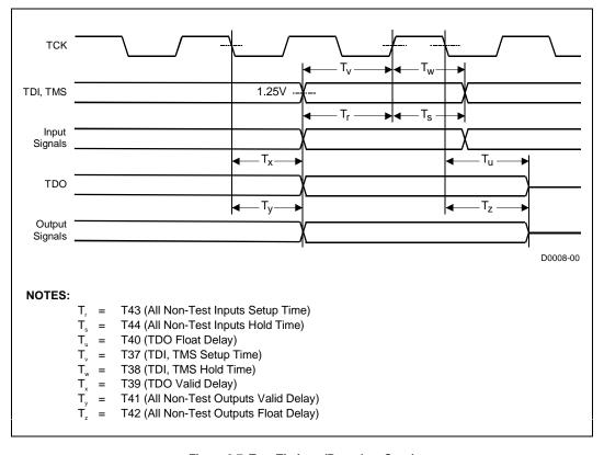
Figure 3.7 Test Timings (Boundary Scan)
