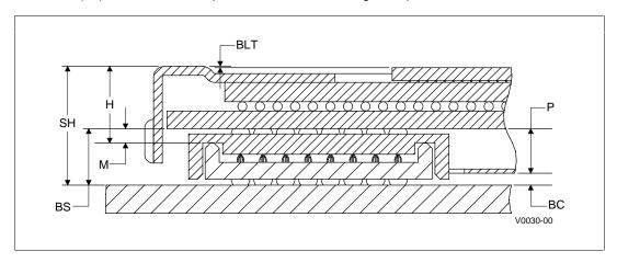
Figure 5.6 Mini-Cartridge Cross-Section with Vertical Dimensions
