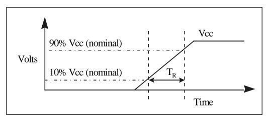
Figure 3.1 Ramp Rate Requirement
