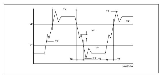
Figure 4.2 BCLK Generic Clock Waveform at the Processor Connector
