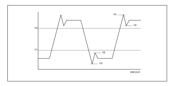
Figure 4.1 BCLK Generic Clock Waveform at the Processor Core
