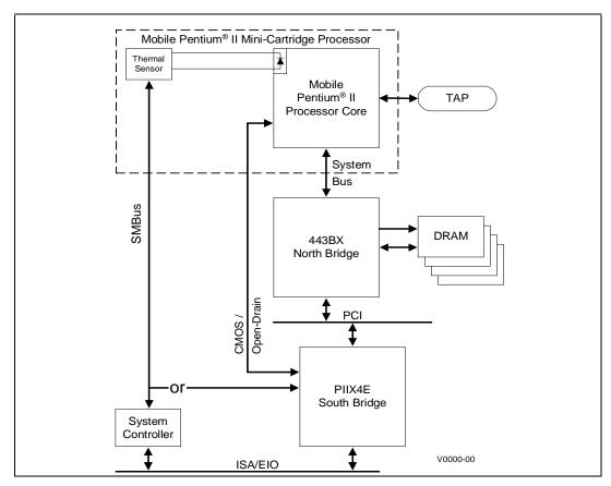
Figure 1.1 Signal Groups of a Mobile Pentium® II Mini-Cartridge Processor-Based System
