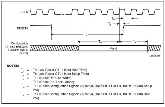
Figure 3.5 Cold/Warm Reset and Configuration Timings
