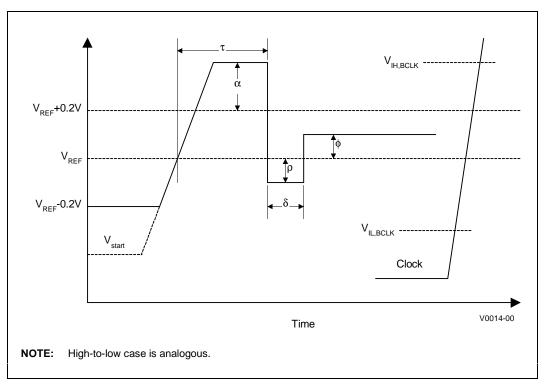
Figure 4.1 Low to High, Low Power GTL+ Receiver Ringback Tolerance
